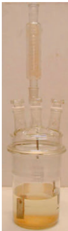
Figure 37.4.1.2: Exposure receptacle with reflux condenser
